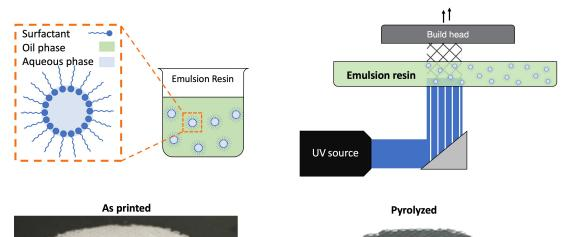
Schematic of novel emulsion stereolithography approach for fabricating lithium sulfide/carbon composite cathodes for Li-S batteries, with images of a 3D architected cathode as printed (polymer/Li<sub>2</sub>SO<sub>4</sub> composite, left) and after pyrolysis (carbon/Li<sub>2</sub>S composite, right).
